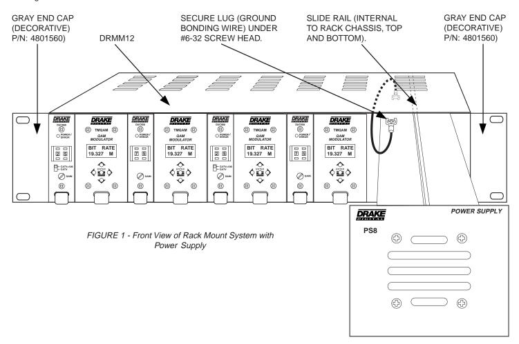
First, install the Drake PS8 Power Supply into the DRMM12. Next, slide individual modules (maximum of 8 units) into the desired rack locations. Connect the DC power cable, supplied with each module, between each module and the PS8 Power Supply.
