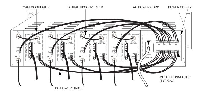
FIGURE 2 - Rear View of System with 4 QAM Modulators and 4 Digital Upconverters.
